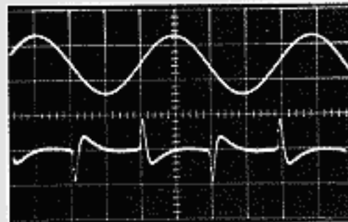
Fig. 2 — 'Scope photo showing the fundamental sine wave (top trace) and a typical crossover distortion waveform (bottom trace).
